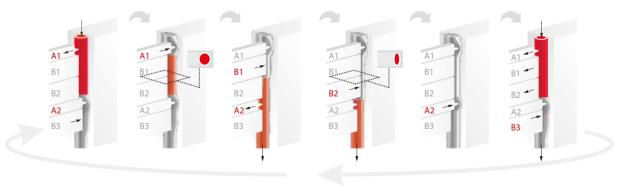
A1 opens, fluid flows into the tube when A2 is closed. A1 closes completely, fluid accumulates in the tube.
